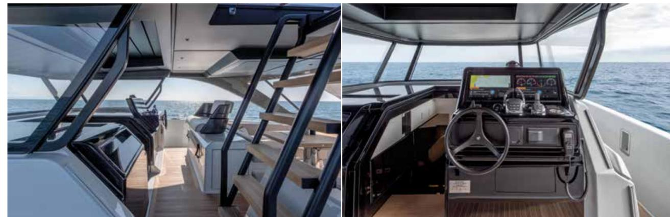
Forward of the cockpit are the ladder to the sunroof, stairs to the lower deck and the helm station, which has a carbon-fibre sofa on top of a locker
